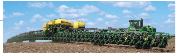
Planter technology has progressed to the point that John Deere is offering a 120-foot machine that can plant 48 rows, each 32 inches apart.
