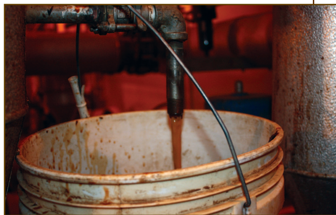
Figure 8. Syrup, or condensed distillers solubles, a by-product of the ethanol distilling process.
