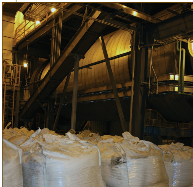
Figure 10. Dryer to dry distillers grains, a by-product of ethanol production.
